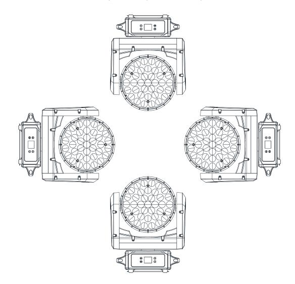
The Vizi Wash Z37 is fully operational in three different mounting positions, hanging upside-down, mounted sideways on trussing, or set on a flat level surface. Be sure this fixture is kept at least 12m (40ft) away from any flammable materials (decoration etc.). Always use and install the supplied safety cable as a safety measure to prevent accidental damage and/or injury in the event the clamp fails (see next page). Never use the carrying handles for secondary attachment.
